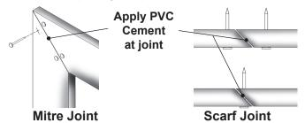
Various adhesives, such as epoxy or polyurethane adhesives may be used to bond our products to other substrates. Consult adhesive labeling to determine suitability.
