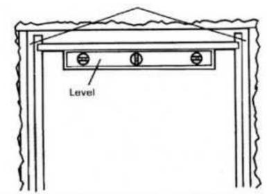
Visually center the top of this frame in the door rough opening. Carefully level the top of the door frame.
